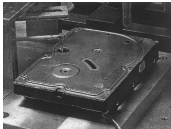
Fig. 10. Experimental setup for ball-bearing spindle; spindle, base, and top.
